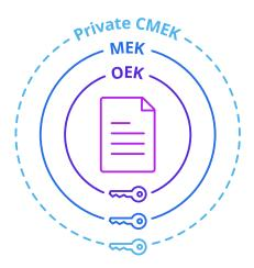
The document is encrypted by the OEK, which is then wrapped by the MEK. If CMEK is active, the MEK is wrapped by the CMEK adding a third layer of encryption to the document.
